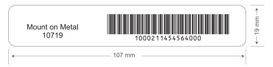
MOM 10719 is a passive UHF RFID label for Mount on Metal applications requiring a narrowest printable tag product. This product is finished with a high performance permanent acrylic adhesive for use on and off metal surfaces. These labels feature a film face to print private logos, product information, or scannable barcodes directly on the label and its additional flexibility for curved surfaces makes it perfect for tracking a variety of transit items.
